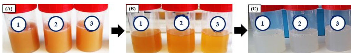
Figure 2.1 — Macroscopic aspect of: (A) initial CGC suspensions in the three NaOH/urea solvent systems; (B) the CGC solutions obtained after removal of the insoluble fraction by centrifugation; (C) the corresponding CGC solutions after dialysis against deionized water. Solvent systems 1, 2 and 3 are represented by the numbers 1, 2 and 3, respectively.
