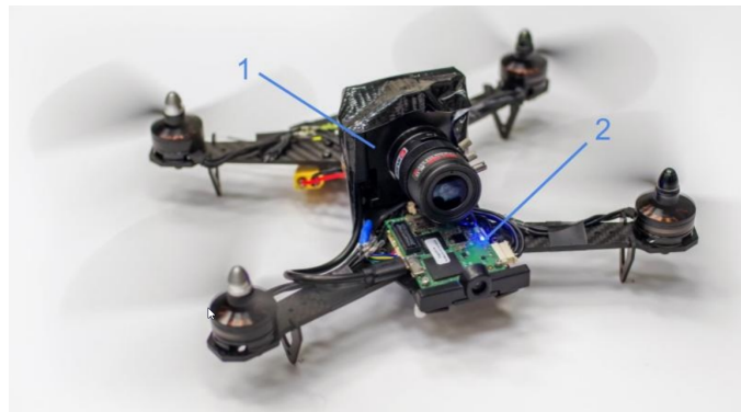
Figure 4.1: Drone used in the dataset collection. 1 – mounted DAVIS240B camera, 2 – customized Qualcomm Flight platform with onboard computer [35].
