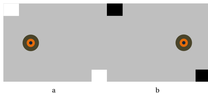
Figure 4.2: Bit "1" in the m-sequence after Manchester and NRZ codification.
