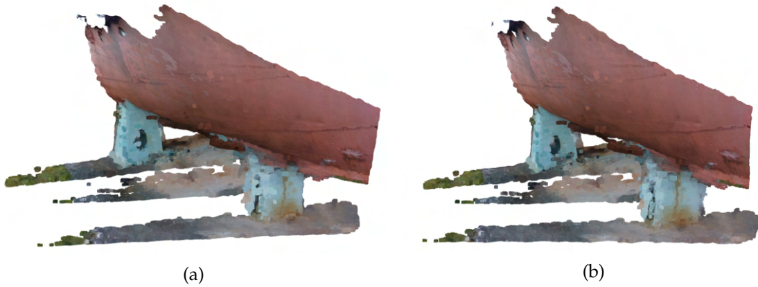
Figure 5.16: Registration of the first point cloud pair of the left side of the ship. a) Fitness Score. b) RMSE.
