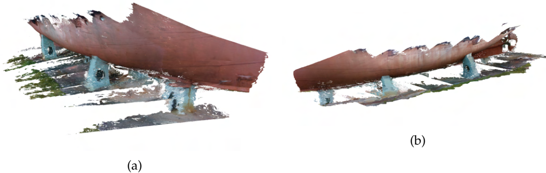
Figure 5.18: Left and right side model of the ship obtained from RGB-D images.
