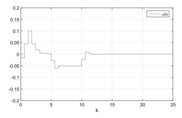
**Fig. 6** Evolution of control signal using the controller in Table 3,  $d_M = 6$  (deviation from the nominal value of the actuator angle  $\theta_a$ )
