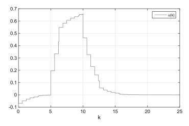
**Fig. 4** Evolution of the control signal using the controller in Table 2,  $d_M = 9$  (deviation from the nominal value of the actuator angle  $\theta_a$ )
