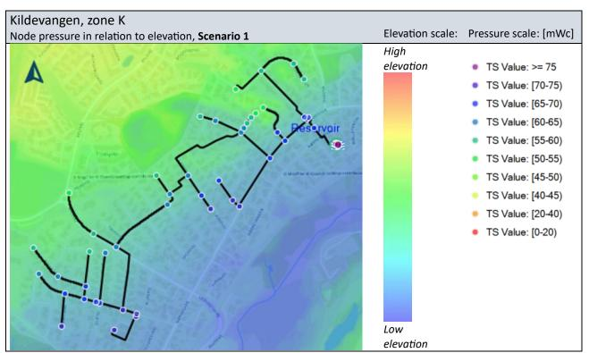
*Figure 8.14 Kildevangen, zone K, node pressure in relation to elevation, Scenario 1*
