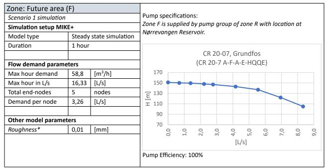
\*A roughness of 0,01 mm has been used which is equivalent to the roughness of new PVC or PE distribution pipes.
