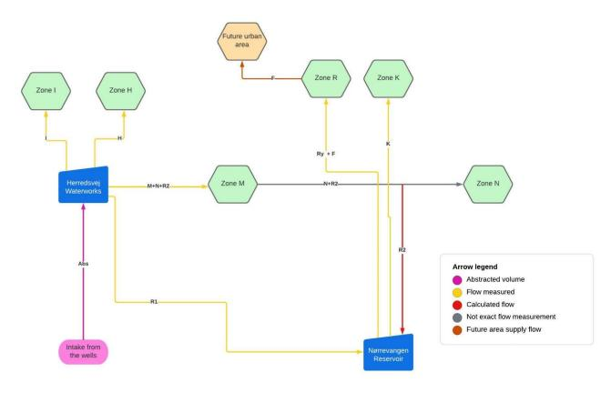
Figure 9.1. Flow diagram for the future distribution system.
