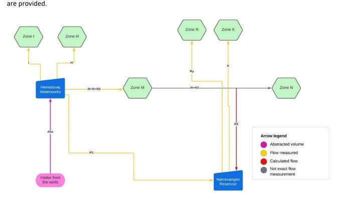
Figure 8.1. Overview diagram of the complete distribution network and denomination of the flows.
