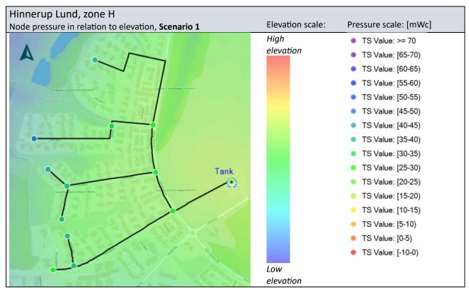
Figure 8.11 Hinnerup Lund, zone H, node pressure in relation to elevation, Scenario 1
