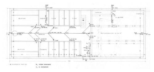
Figure 7.11 Schematic drawing of the floor plan in the Hinnerup waterworks. The drawing is not quite up to date, the "Dosering" has now also been converted into a sand filter.
