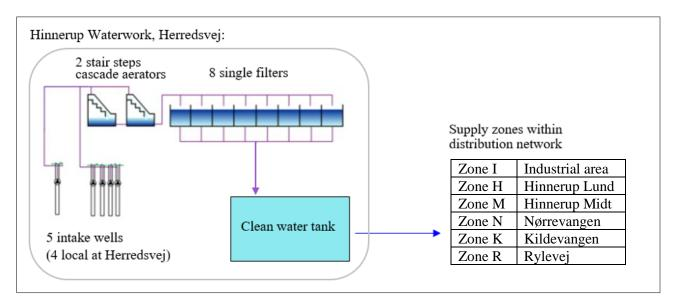
Figure 5.4 Simplified diagram overview of the complete supply system of Hinnerup.
