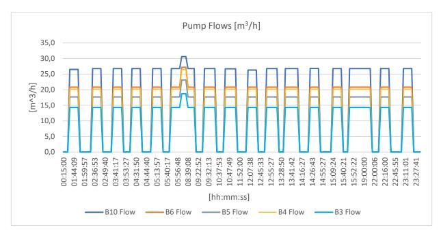
Figure 10.1. Abstraction pumps flow during a 24h period.
