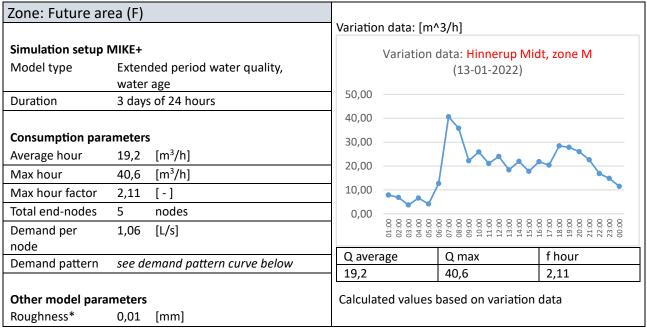
\*A roughness of 0,01 mm has been used which is equivalent to the roughness of new PVC or PE distribution pipes.
