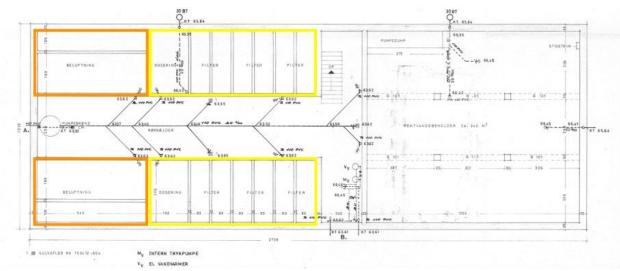
Figure 7.6 Schematic drawing of the floor plan in the Hinnerup waterworks. The orange marked areas are the Cascade aeration. In yellow the Sand filters can be seen. The drawing is from 1973. Since then, the "Dosering" has now also been converted into a sand filter. Provided by the waterworks.
