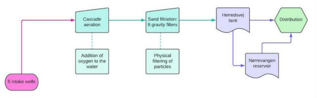
*Figure 7.4.* Overview diagram of the standard treatment and the way to the distribution system in Hinnerup.
