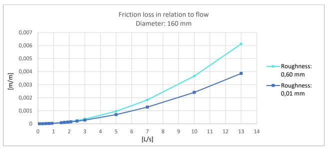
Figure 8.10 Friction loss in relation to flow at different roughness, diameter of 160 mm.
