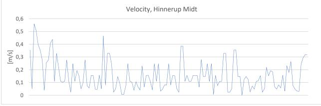
Figure 8.25 Variation in velocity within network, zone M
