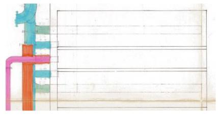
Figure 7.8 The top view of one of the eight sand filters in Hinnerup showcases color-coded pipes entering and exiting the filter. The raw water flow is indicated by the color red, the clean water flow is marked in blue, the backwash water is represented by green, and the pink pipe is used for air ventilation during the backwashing process. Excerpt from drawing provided by the waterworks.
