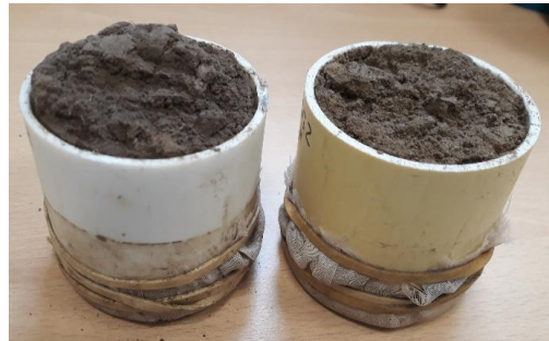
Figure 2. Soil samples with two coupled cylinders, which were used to access roughness at a depth of 5 cm.
