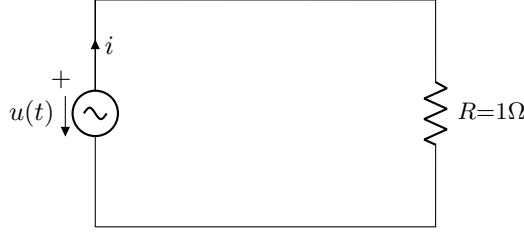
Figure 2: Resistor load and non-sinusoidal source
