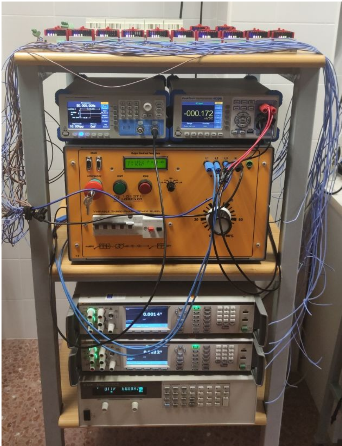
Figure 8: Equipment used to calibrate 3Ph-oZm: On top, some 3Ph-oZm's prepared to be calibrated. DL 1013T variable three-phase power supply is shown in yellow box, while two 8.5 digit high accuracy multimeters Fluke 8558A and an Agilent 6812 digital power supply are located at the bottom.
