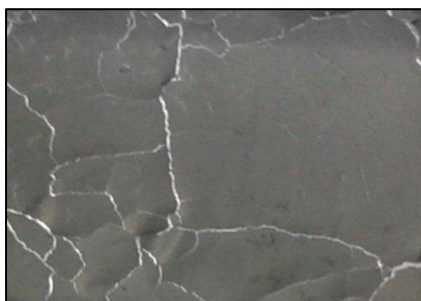
Fig. 45 Catalyzed carbon film on the surface of pure liquid Ga.
