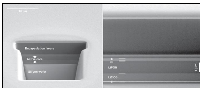
Fig. 17 FIB/SEM cross-section of a thin film encapsulated LIB comprising the Li 1.2 TiO 0.5 S 2.1 /LiPON/Si active layers and titanium current collectors [147].
