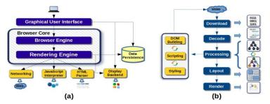
Fig. 3. Web Browsers Reference Architecture and Rendering Engine.
