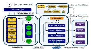
Fig. 4. Browser Architecture Core Components.
