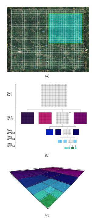
Figure 2. Construction of a TGPT from an arbitrary ROI and its posterior usage for computing the different levels of detail of the image. (a) Illustration of an ROI defined by user (inner shaded rectangle, overlapping  $16 \times 18$  tiles) over a dataset grid (outer rectangle,  $32 \times 39$  tiles). (b) TGPT structure generated during the multi-resolution process fitting the ROI shown in (a). (c) Point cloud rendered by *ViLMA* obtained from the TGPT shown in (b).
