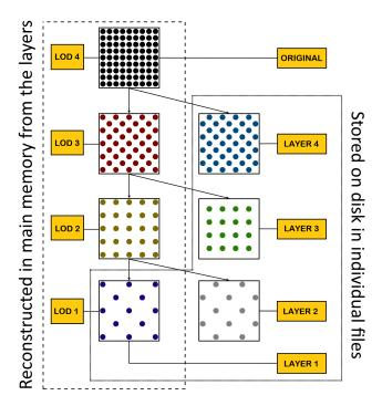
Figure 3. Layer generation of a single tile carried out during the *Preprocessing Stage*. Starting with the original point set (upper square) four layers are generated (labelled squares).
