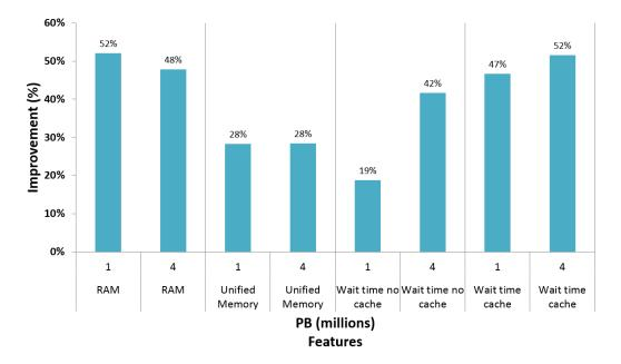
Figure 8. Performance comparison between loading the full dataset of *PNOA* and loading only an ROI from it.
