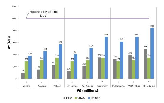
Figure 5. RAM, VRAM and Unified memory (RAM + VRAM) consumption during the performance tests for different point budgets.
