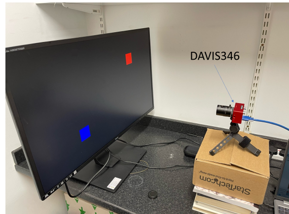
Fig. 2. The setup used to collect EACC data (this does not reflect the true capture conditions which were automated, in a darkroom with no human attendance).
