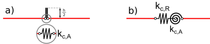
Figure 13: Connection spring models: a) axial spring with lever arm; b) series of rotational and axial non-dimensional spring
