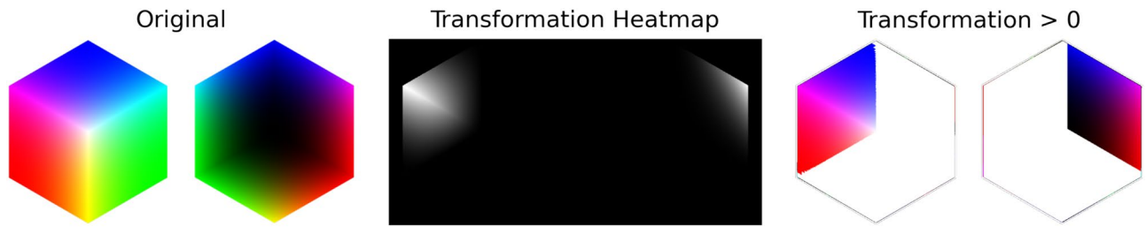
Figure 2. Left: Two 24-bit colour cubes, one with the white corner at the origin and one with the black corner at the origin. Middle: The values of the pixels in the representation specified in Eq. 1 and Alg. 1. Right: The pixels that have values greater than 0 in this representation.
