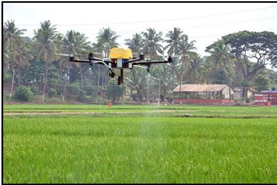
Figure 2.1: Hexacopter spraying pesticides in Tamil Nadu Agricultural University Farm rice fields in Tamil Nadu, India, during October 2019.
