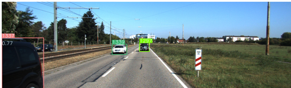
(a) The model is able to identify all the moving cars in the image and ignores the parked car
