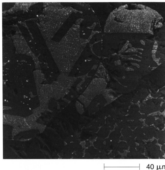
Figure 10. BSE micrograph of two smaller silicon spheres beside the initial silicon sphere.
