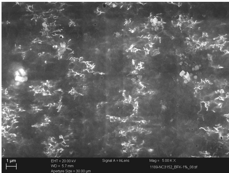
Fig. 10. SEM-CCI images of the PA12 composite with 1 wt.% Nanocyl™ NC3152 and 1 wt.% BCA .
