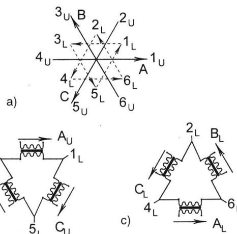
Figures 11a to c. Diagrams used as aids in designing VEM's, a) phasor diagram constructed while developing an electrically symmetrical melter with 12 electrodes. Solid lines are the applied cross-fired voltage phasors for the upper set, dashed lines are the applied delta-fired voltage phasors for the lower set; b) delta-connected secondaries for electrodes no. 1, 3 and 5 of the lower set; c) delta-connected secondaries for electrodes no. 2, 4 and 6 of the lower set.
