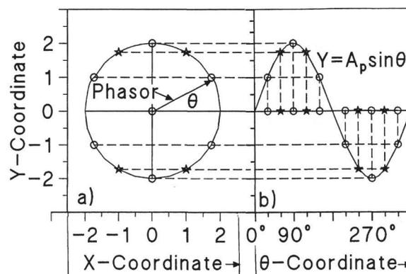
Figures 18a and b. Construction of a sinusoidal wave using a phasor, a) angular positions of a phasor (adjusted to the peak value of the sinusoid) used to construct a sine curve; b) sine curve generated by the counter clockwise rotation of this phasor.
