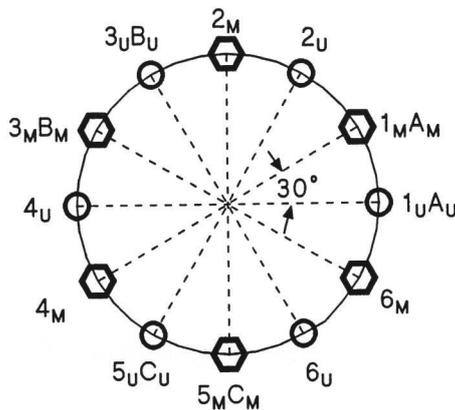
Figure 8. Electrode positions and voltage connections for a VEM with an upper (U) and a middle (M) tier of electrodes off-set by 30°. Letters A, B and C indicate relative connections and will correspond to the heads of the respective applied voltage phasors.
