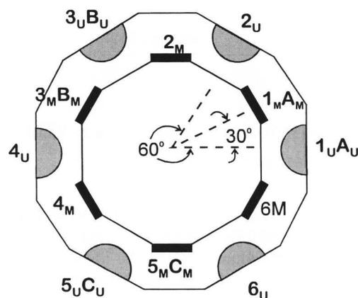
Figure 10. Sketch, top view of a two-diameter Vertical Electric Melter showing inside contour and differently shaped electrodes.
