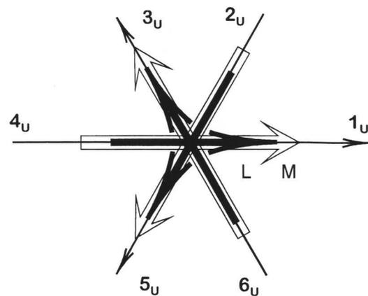
Figure 6. Phasor diagram for a symmetrically built, cross-fired VEM with an increased voltage ( $V_{4U-1U}$ ) in phase A of the top tier, thus making the electrical distribution asymmetric. Note that phasor  $A_{(4U-1U)}$  is longer than the others.
