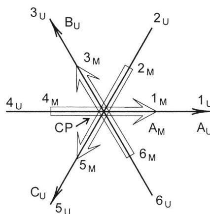
Figure 9. Phasor diagram for a cross-fired melter with level 1 and 2 electrodes off-set by  $30^\circ$ . Drawn with  $V_U/V_M = 2$ .
