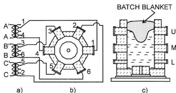
Figures 1a to c. Cross-fired, vertical, electric melter (VEM) with in-line electrodes, a) three-phase power supply; b) horizontal cross-section of a cross-fired S-VEM; c) vertical cross-section of a S-VEM showing electrodes and central outlet.
