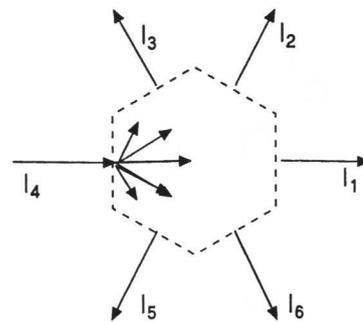
Figure 5. Line current phasors and components.  $I_4$  is for a cross-fired S-VEM (no scale).
