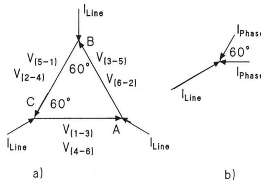
Figures 16a and b. Current and voltage phasors for a symmetric unit wired per figure 15, a) applied voltage and line current phasors showing "pure" peripheral firing, i.e. no electric currents between diametrically placed electrodes; b) representative line and phase current phasors.
