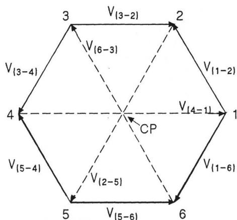
Figure 13. Applied peripheral voltage phasors (solid lines), resultant cross-fired voltage phasors (dashed lines).
