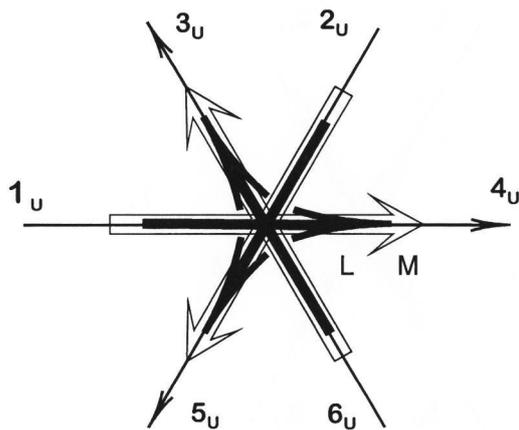
Figure 7. Phasors for a 3-tier, cross-fired VEM with leads to electrodes no. 1<sub>U</sub> and 4<sub>U</sub> reversed. Note interchange of electrode numbers 1<sub>U</sub> and 4<sub>U</sub> on phasor A.
