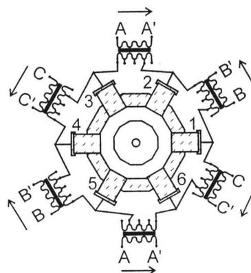
Figure 12. Plan view of a S-VEM and a 3- $\phi$  circuit for peripheral heating.
