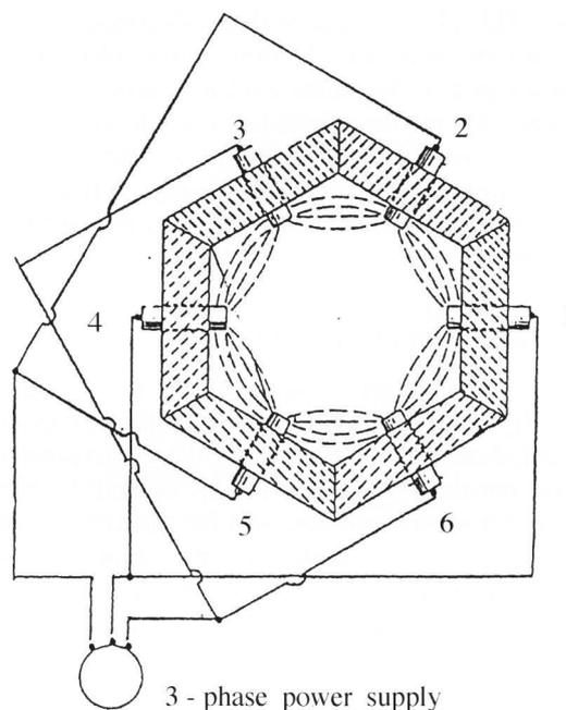
Figure 15. S-VEM with "pure" peripheral heating, i.e. with no cross-fired components.
