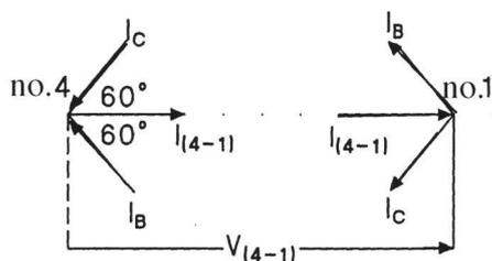
Figure 14. Current phasors for electrodes no. 4 and 1 of figure 13 with applied peripheral firing.
