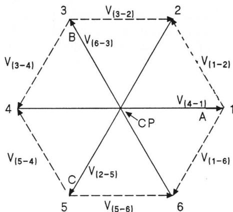
Figure 3. Applied (line) voltage phasors (solid lines) for the physically symmetrical, vertical melter (S-VEM). Dashed lines around the perimeter are the resultant (peripheral) voltage phasors between adjacent electrodes.
