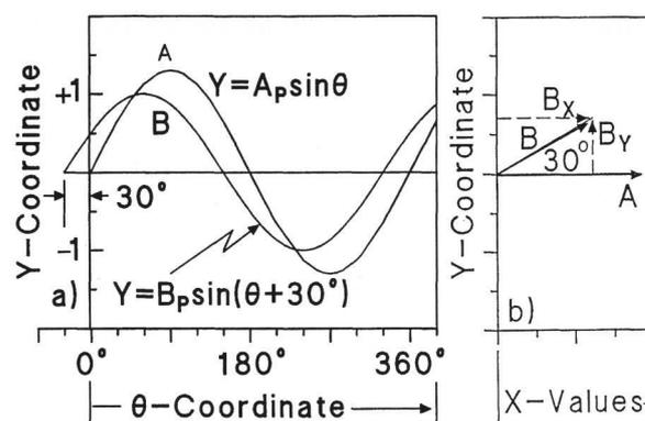
Figures 17a and b. Relations between two sinusoidal curves, a) curve A lags curve B by a phase angle  $\beta = 30^\circ$ ; b) phasor representation of the two sinusoids. Note that the phasor for curve A lies along the  $x$  axis so its  $y$  component is equal to zero:  $B_x$  and  $B_y$  are the  $x$  and  $y$  components of phasor B.
