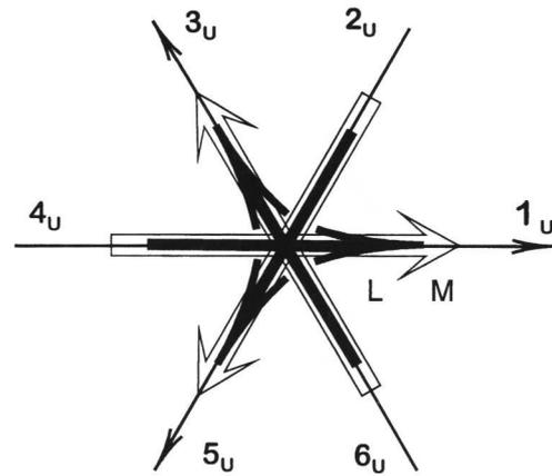
Figure 4. Upper, middle and lower circuit phasors for the cross-fired S-VEM with decreasing voltages top to bottom.
