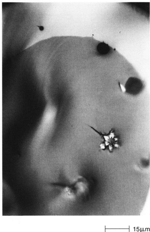
Figure 12. Optical micrograph of a fracture surface of fiber and overclad.
