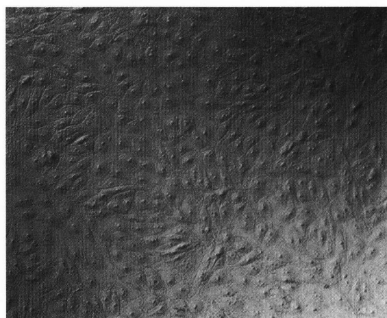
Figure 2. Bright-field Nomarski interference contrast micrograph of cellular monolayer (MDCK) on the surface of the sputtered layer.
