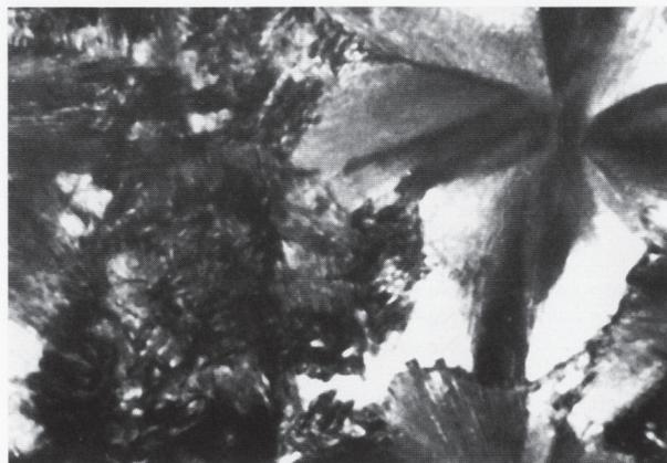
Figure 2. Photomicrograph of 1.5 wt% LiF-containing glasses heat-treated at 900°C for 4 h: fair-sized fibrillar spherulites enveloped by bundles of fine nepheline crystals and some interstitial residual glass in-between.
