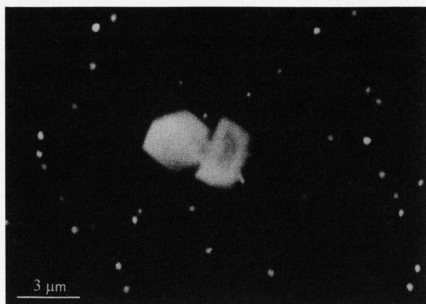
Figure 4. Sample AA2: BSE image of hexagonal inclusions of chromium spinel and minute spherical inclusions of an iron-sulphur phase.
