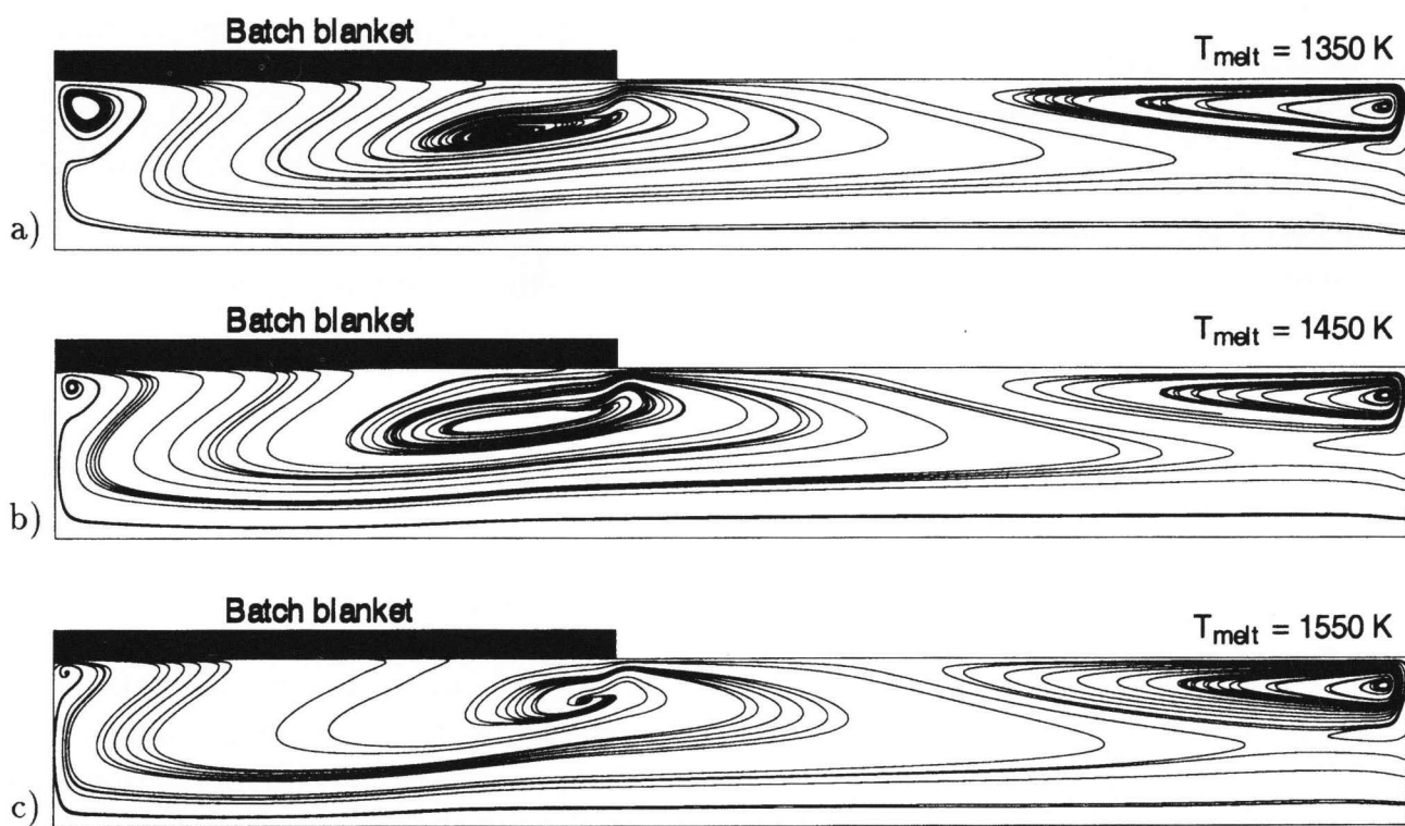
Figures 4a to c. Effect of T_{\text{melt}} on the streamlines at the midplane for a) T_{\text{melt}} = 1350 K, b) T_{\text{melt}} = 1450 K, and c) T_{\text{melt}} = 1550 K.
