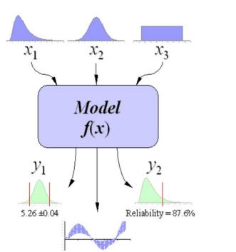
Fig. 3. The simple principle of the Monte Carlo simulation [9]
