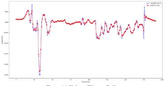
Figure 16. Kalman Filter on Roll
