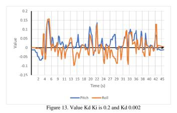
The results obtained from the gyroscope output show that the response received is more unstable than the Kp and Ki tests of 0.05.
