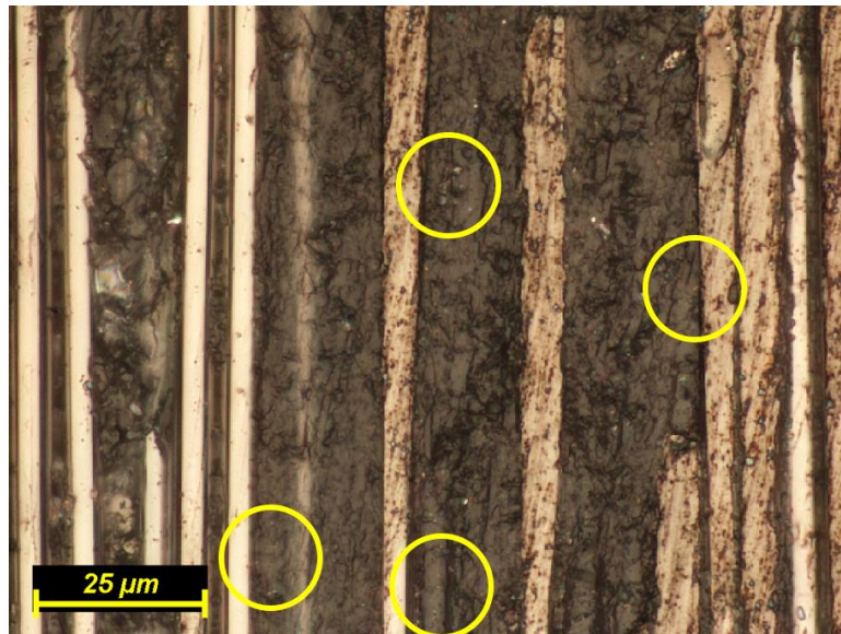
Figure 26: Image of 4 plied T700s 1wt% CNF ZTCFRP, 1000x. The yellow circles show the CNF facing the Z-direction perpendicular to the CF direction.
