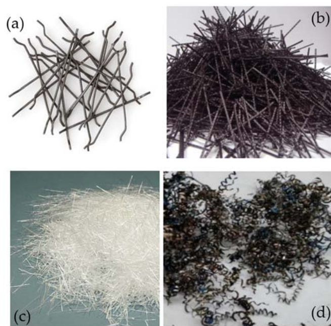
Figure 2. Fibres used in this study. (a) Low carbon steel fibres; (b) Modified polyolefins fibres; (c) 12 mm and 36 mm glass fibres; (d) Lathe waste fibres.
