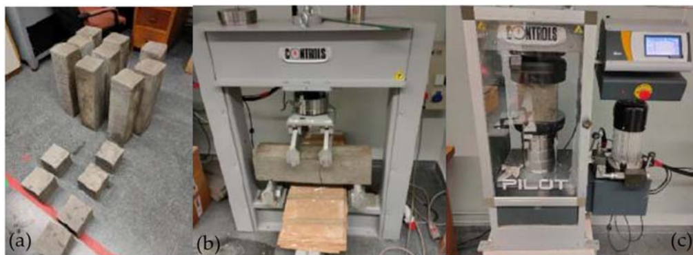
Figure 3. (a) Test specimens. (b) Flexural test. (c) Compression test.
