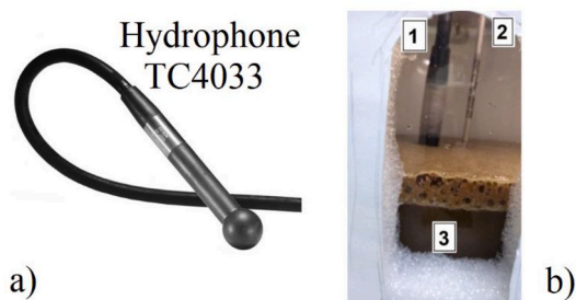
Fig. 1. (a) Hydrophone TC4033. (b) Photography of the fermenting liquid and sensors location through the inspection window of the 8 L experimental reactor. 1-Hydrophone, 2-Type-J thermocouple sensor, 3-Fermenting liquid (after 24 h).
