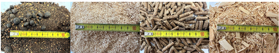
Figure 3. Examples of different biomasses: (a) pomace, (b) malt dust, (c) olive pellets, (d) wood chips.
