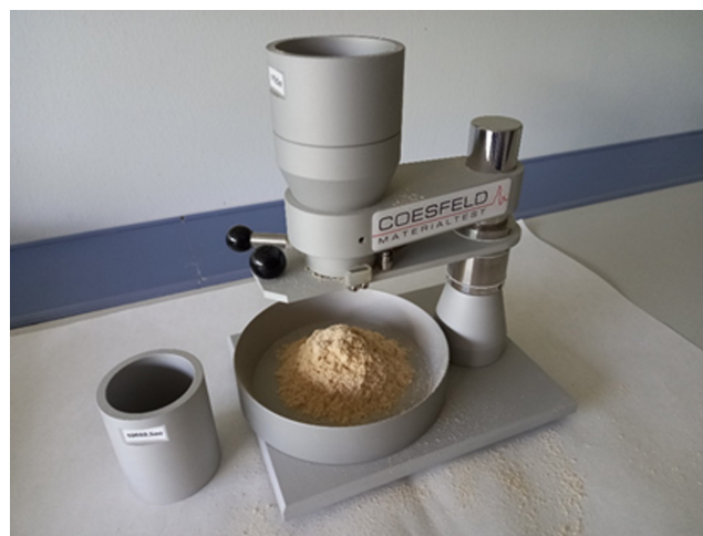
Figure 3. Apparent density tester used to determine the angle of repose. The picture shows the pile of sample S-3 (<400 \mu\text{m} ) on the base plate after discharge. On the left, the 100 mL container used for the bulk density measurements.
