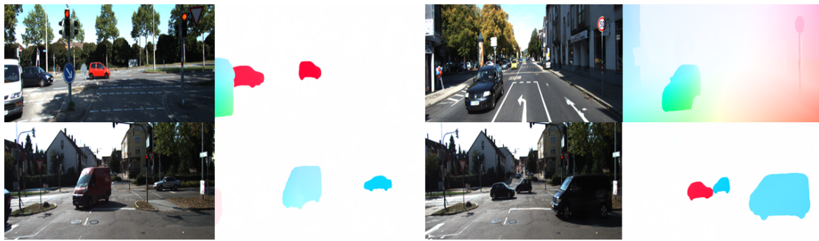
Figure 4.1: Sample frames from KITTI2015 test dataset and their corresponding optical flow estimates using our SSTM method.
