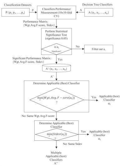
Fig. 4 Multi-criteria analysis for algorithm performance evaluation
