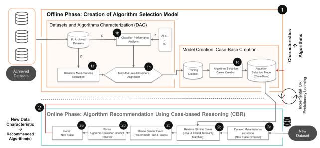
Fig. 2 Case-based reasoning for algorithm selection
