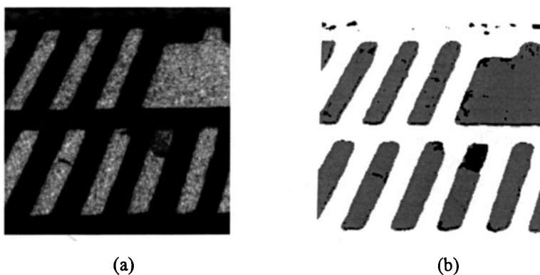
Figure 8. (a) Input SAM image with incomplete metallization (b) Segmented image
