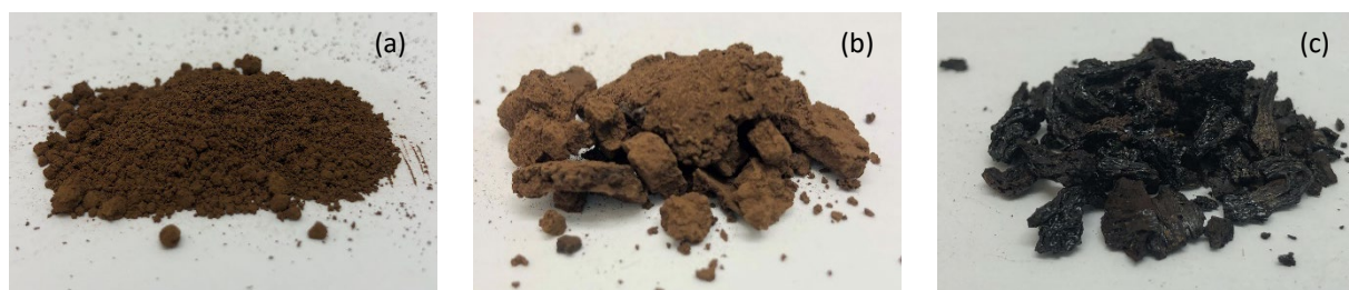
Figure 10. Solid product from solvent liquefaction of lignin are markedly different for the two reactor systems; (a) Raw lignin after ball milling; (b) solid product from the SBA after 0 minutes of nominal reaction time resembles original lignin; (c) THF-insoluble solids from ICBA reactor after 0 minutes of nominal reaction time resembles char.
