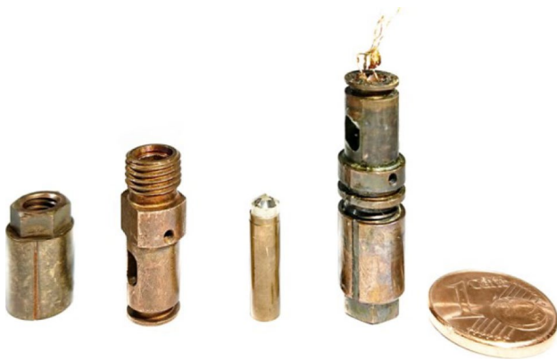
Fig. 3 The design of the miniature nonmagnetic DAC. A photo of the assembled miniature DAC (right) and its parts (left)
