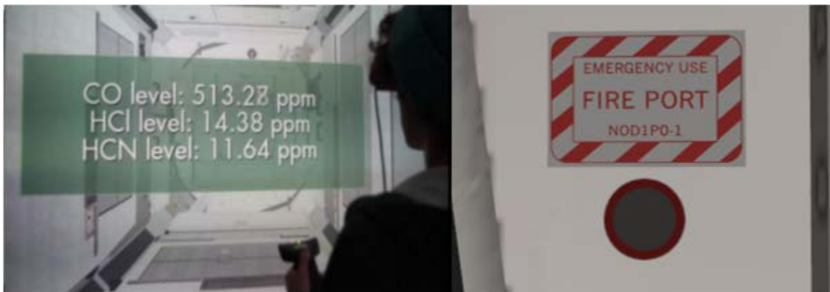
Figure 3: The CSA-CP in the VRE displays environmental noxious gas readings (left) and fireport with identifier code (right).
