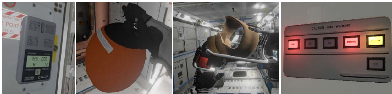
Figure 3: VR-ISS emergency fire equipment, (A) Compound Specific Analyzer-Combustion Products, (B) Portable Fire Extinguisher, (C) Portable Breathing Apparatus, and (D) Caution & Warning Panel.
