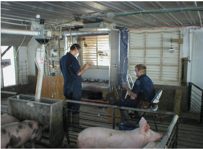
Figure 4. Fan calibration process at the Texas site.
