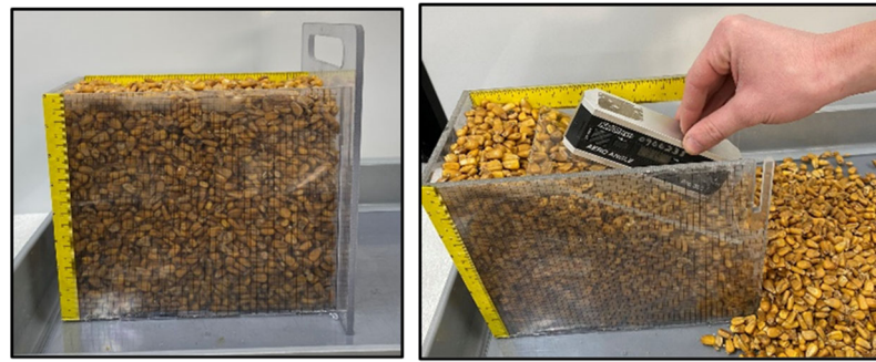
Figure 6. Grain filled discharge container ( left ). Measuring the angles of repose for discharged grain after the gate has been removed ( right ).
