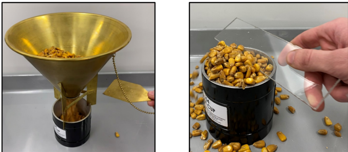
Figure 1. Grain emptying into container from discharge funnel (left). Leveling the contents with straight edge per USDA standard instructions [17] (right).
