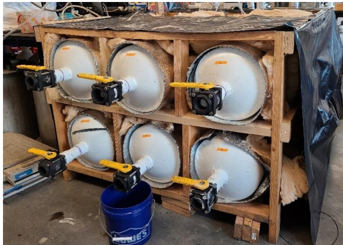
Figure 2. Picture of six 100-L anaerobic digesters in placed
