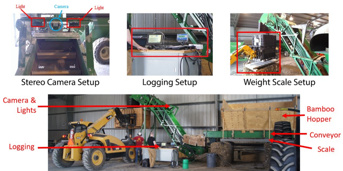
Fig. 1 A picture of the overall system showing the laboratory setup for volume measurement testing.
