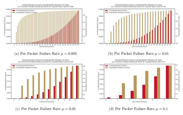
Figure 15: A comparison of the impact on differing numbers of data packets per burst on the percentage of bursts with untolerated failures, and the percentage of bandwidth utilized for productive data transfer for per packet failure rates of  $\mu \in \{0.005, 0.01, 0.05, 0.1\}$
