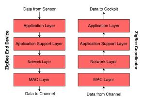
Figure 8: Abstracted and layered ZigBee communication network model showing data flow across layers.
