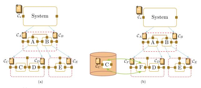
Figure 2: (a) Component hierarchy in a compositional system. The system is composed from components A and B. Component A is composed from component C and D, and component B from component E. (b) Contract-based design allows easy re-use of components from a library provided the contracts of the swapped components are the same.
