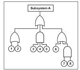
Figure 3: A sample fault-tree that uses Boolean logic to combine low level events that lead to an undesired state of a system
