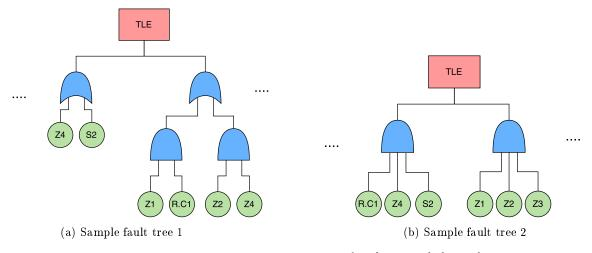
Figure 12: Fault tree using minimal cut sets for the extended wired system.
