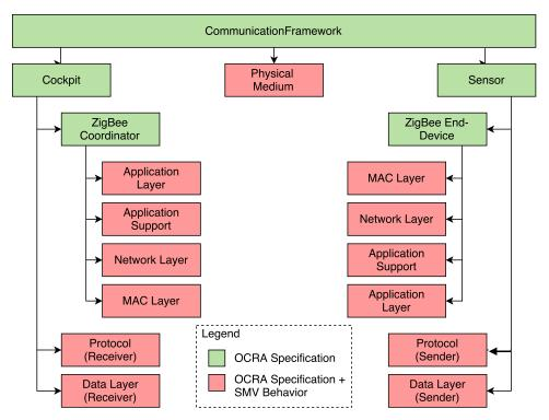
Figure 9: Nominal framework model for the ZigBee wireless communication system
