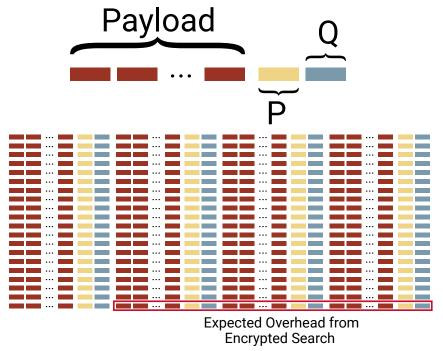
Figure 5: Anatomy of a file transmitted using secure, and reliable, packet bursts. Each burst consists of an adjustable number of payload packets carrying data or meta-data, and parity packets. Extra encrypted search meta-data is included in additional bursts. The example in the diagram represents the expected proportion of extra bursts that must be transmitted to implement searchable encryption mechanisms.
