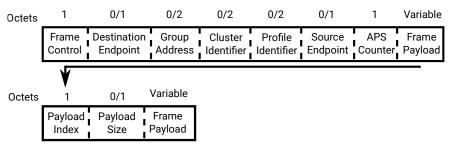
Figure 6: Modified format of ZigBee packet as part of a burst.
