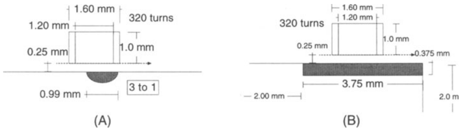
Figure 4. Illustration of the dimensions of the equivalent coil and the cracks. (A) is for the flat-surface crack, which is semi-elliptical of the length 0.99 mm with the aspect ratio 3 to 1. (B) The edge crack is a rectangular EDM notch. The coil parameters are determined empirically from the flat-surface data (Fig. 5A below). See the text for details.
