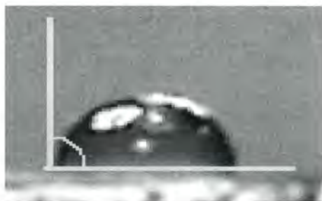
Figure 18. Example of contact angle measurement.
