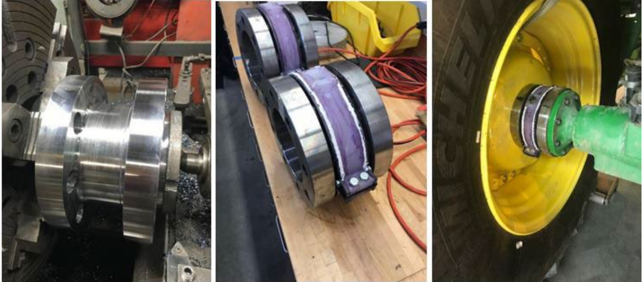
Figure 2. Wheel spacer torque sensor consisted of the spacer after Lathing process (left), strain gauge and protective cover installation (center), and torque sensor mounted to the rear wheel of the tractor (right).
