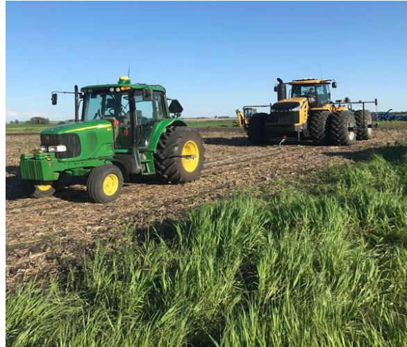
Figure 4. 2WD test tractor attached to 4WD load tractor.
