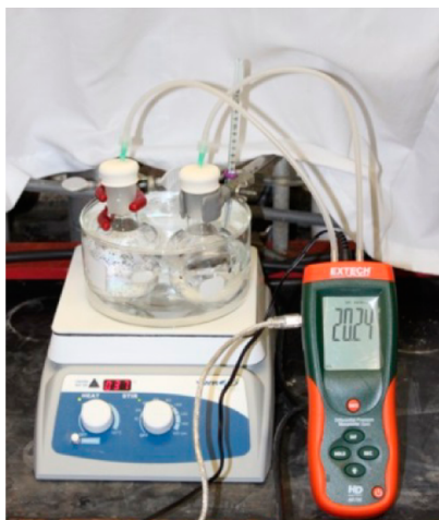
Figure 8. Experimental setup for monitoring pressure from O_2 evolution during H_2O_2 decomposition accelerated by the PNU-MFC catalysts. (Left) Constant temperature water or ice bath holds working and control round-bottom flasks on a hot plate while (right) a differential pressure monitor measures pressure changes. A USB cord (silver) originating from the differential pressure monitor connects to a laptop monitor for data analysis.
