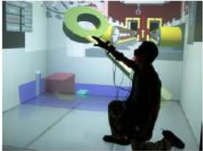
Fig. 7 Data Glove in a Six-Sided CAVE
