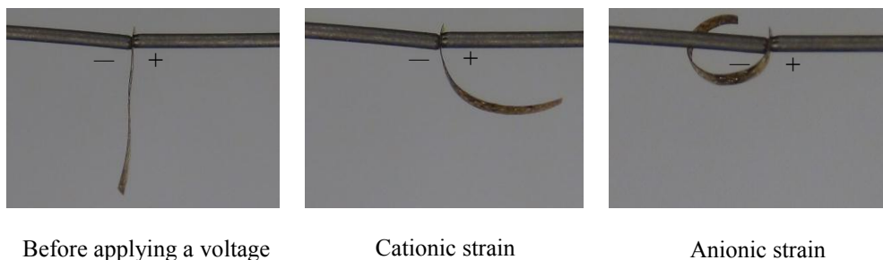
Fig. 2.8 Photographic images of an IPMC-based actuator with 30 bilayers of AuNPs/PAH in CNC; electrode on the right side is anode.
