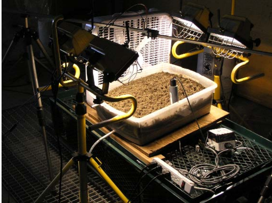
Figure 1. Experimental set up for drying the soil and collecting moisture and spectral data
